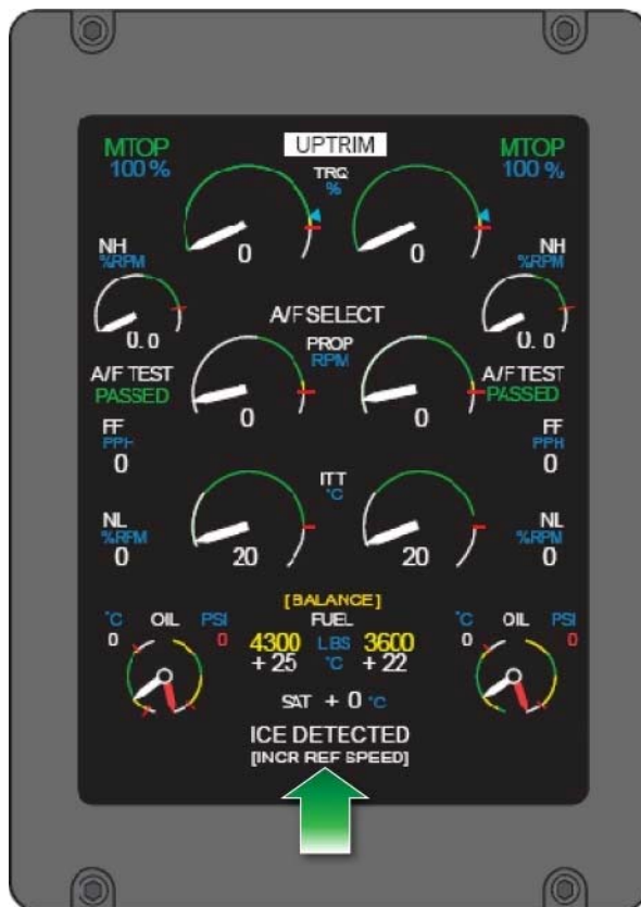
Figure 3. Q400 Engine Display Showing Ice Detected and Increased Reference Speeds Message
