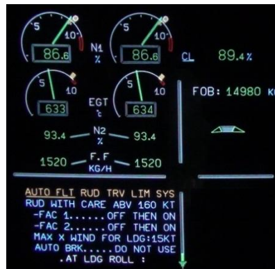
Figure 34: The ECAM messages after RTLTLU 1 and 2 fault
