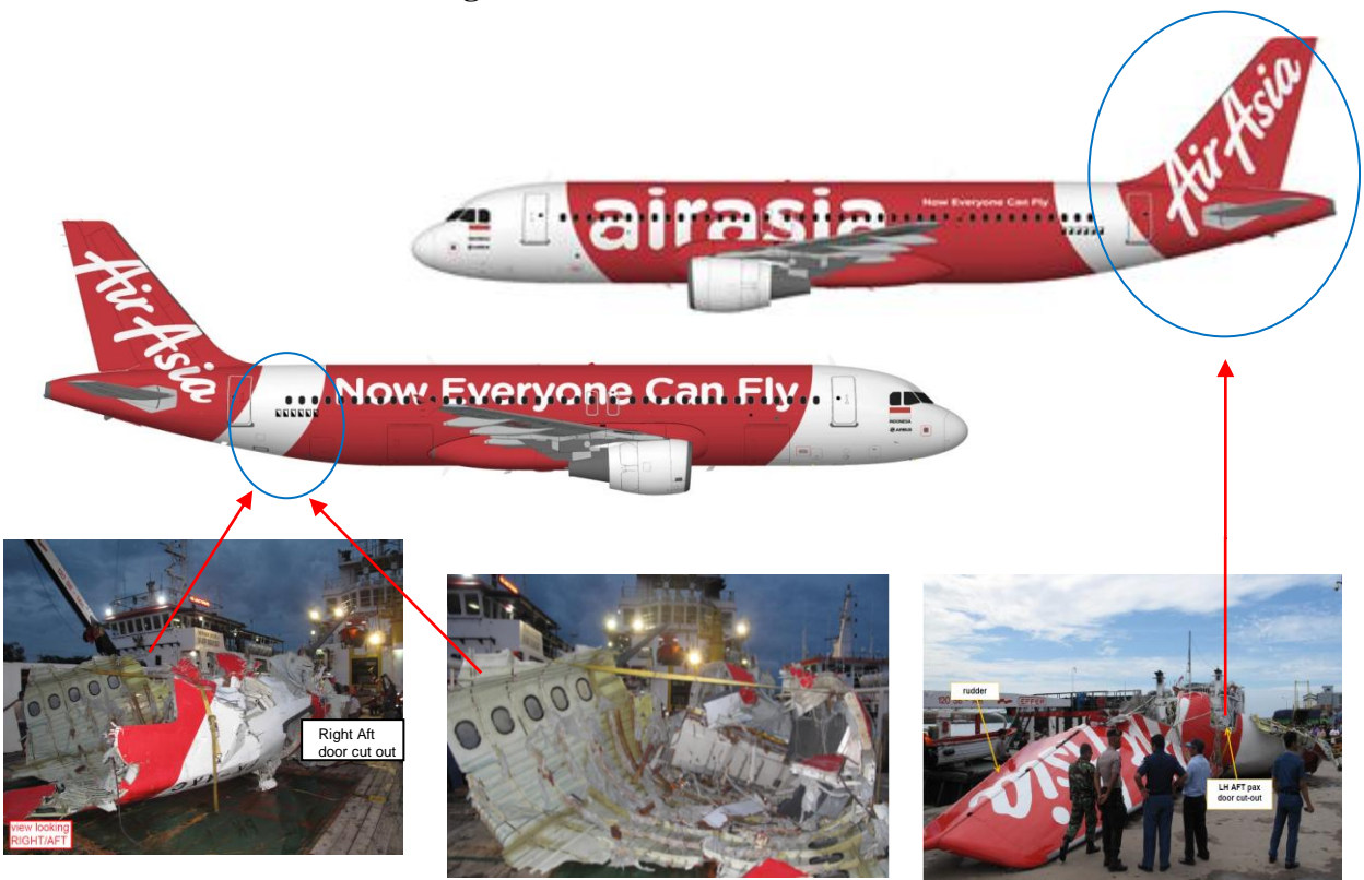
Figure 32: Pictures of identified parts and its original position
